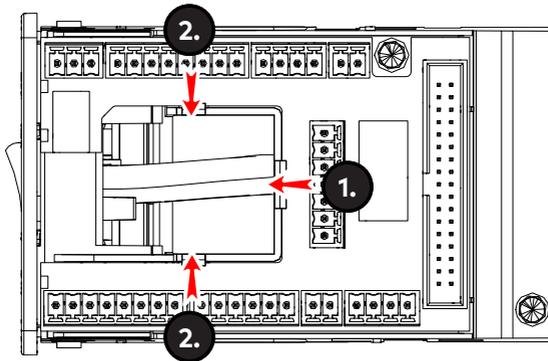
7. Insert the cable ends of the connection cables from the inside to the empty board slot.
